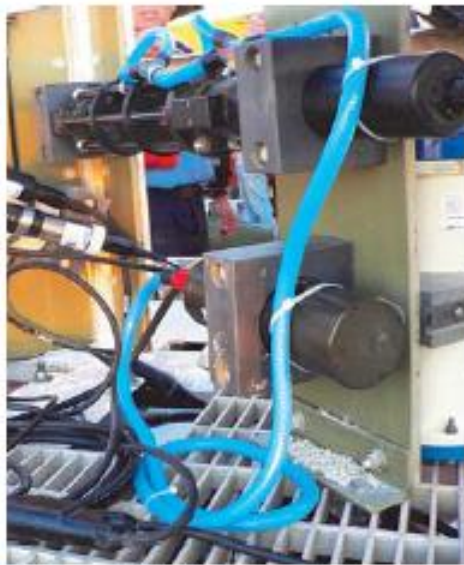
Figure 4. IFREMER Biofouling system on VENUS
